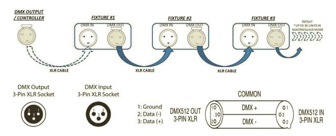
For installations where the DMX cable has to run a long distance, or is in an electrically noisy environment, it is recommended to use a DMX terminator. This helps in preventing corruption of the digital control signal by electrical noise. The DMX terminator is simply an XLR a 120 120  $\Omega$  resistor connected between pins 2 and 3, which is then plugged into the output XLR socket of the last fixture in the chain. Please see illustrations below:
