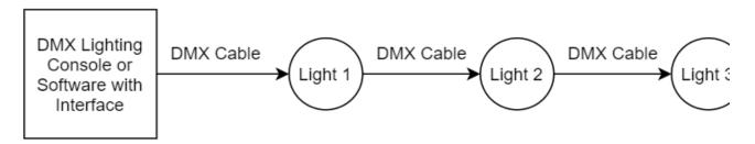
**32 Fixture Rule** – DMX only allows you to connect up to 32 fixtures in a single daisy chain for signal strength. Sometimes, depending on the fixtures and cable length, this number is less (or more).
