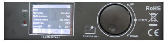
Notice:You can touch the Touch screen or rotate the round button to select the functions(rotate the round button=UP/DOWN,press the round button=ENTER).
