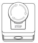
Connect the optional remote-control safety switch to the corresponding socket of the device. If you press the switch, the laser beam will be switched off immediately. To unlock the switch and resume operation, turn the knob clockwise.
