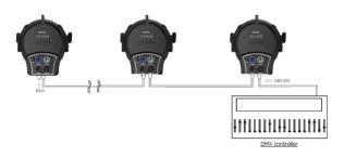
Connect the DMX-output of the first fixture in the DMX-chain with the DMX-input of the next fixture. Always connect one output with the input of the next fixture until all fixtures are connected. Up to 32 fixtures can be connected.
